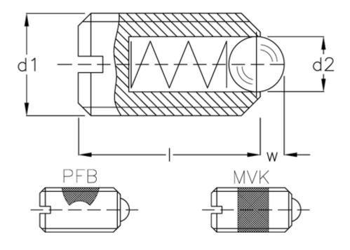
$\begin{array}{ll} \text{d1} & = \text{M16} \\ \text{d2} & = 10.0 \\ \text{Length I} & = 24 \\ \text{Spring pressure N bottom} = 86.0 \\ \text{Spring pressure N top} & = 41 \\ \text{W} & = 3.5 \end{array}$
